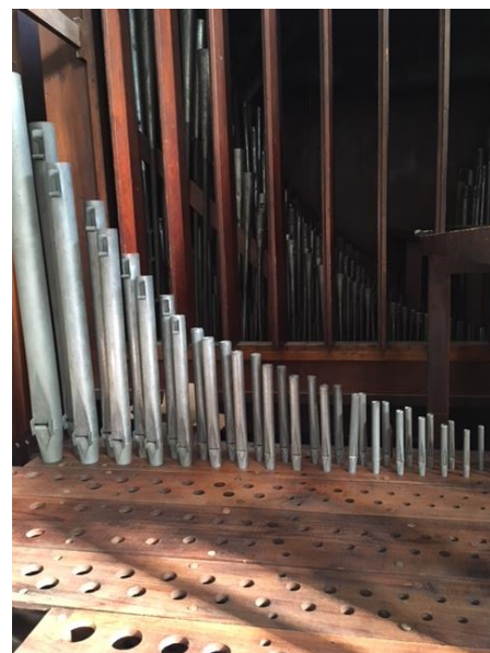
Restored pipes going back into their newly cleaned home on the wind chest. These are the 4' Great Principal pipes.
